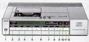
14 PROGRAM(me) display: a LEDbar display which indicates the num- an operating or programming error. ber of tracks on a disc; also used as an aid in compiling a programme. 15 TRACK display: a LED-bar display in which the LEDs light one at a time to indicate the track in play; also used to locate tracks for programming.
