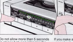
Do not allow more than 5 seconds to elapse between releasing the CANCEL key and pressing the SELECT key to make the next selection, otherwise the TRACK Display LED will go out. It will flash again if you press SELECT once more, but then under the first LED of the PROGRAM Display. This, however, does not affect the tracks that have already been cancelled from the memory - they remain cancelled - and you can move the TRACK Display LED on to the next track you want to cancel.
